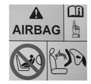
The Airbag Warning Symbol on sun visor reminds extreme hazards associated with the use of rearward-facing child restraint on front passenger seat during airbag deployment.
