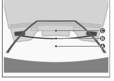
Visually check the surroundings and the area behind the vehicle. On the screen, it appears that a truck is parked at point B. However, in reality if you back up to point A, you will hit the truck. On the screen, it appears that A is closest and C is furthest away. However, in reality, the distance to A and C is the same, and B is further away from A and C.
