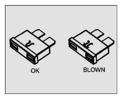
· Remove the blown fuse by "fuse
