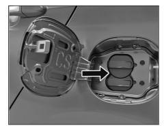
7. Before connecting the charging gun to vehicle charging socket, make sure the gun lock is released.
