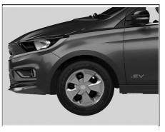
Put a piece of cloth between the spokes of the wheel cover and pull it outwards. Take out detached wheel cover from the wheel rim.
