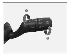
Inner rotary switch on right hand stalk is provided for head lamp leveling. With the inner rotary switch, Head lamp leveling can be done with head lamp in Low Beam and in 'ON' position. Select correct position before start of trip, when the vehicle is stationary. Depending on the number of passengers and luggage in the vehicle headlamp focus may change. This can be adjusted by rotating the knob to one of the three level positions.
