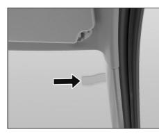
Tag holder is provided near the front windshield for ease of displaying toll, parking tickets, ID's, passes, labels etc.
