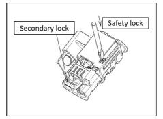
Secondary lock need to be opened and then safety lock to be pulled with suitable tool.  After successfully completion of service, press the secondary lock inside and safety lock to its original position.
