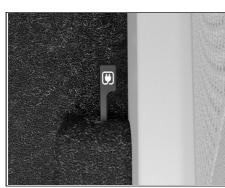
To release the Charging port flap, pull the lever located at the right hand side below the driver seat.
