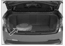
• To remove the spare wheel, unscrew and remove the retaining bolt.
