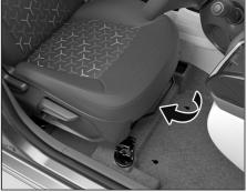
The jack is placed under the driver seat.
