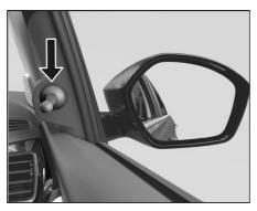
You can adjust the outer rear view mirror manually by joy stick knob located in the driver's and front passenger's door panel.
