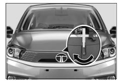
4. Lift the bonnet up. Pull the bonnet stay rod from its clip and engage the free end into the slot.
