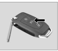
Press and hold approach light button for few sec until the tailgate is unlock.
