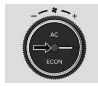
In-car sensor on HVAC control panel.
