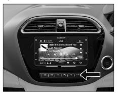
To open the tailgate press the switch located on fascia switch. Flip Key (if equipped)
