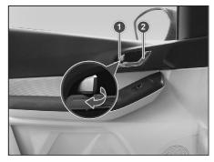
All the doors can also be locked from inside by pressing knob (1) on driver door and independently on other doors respectively.
