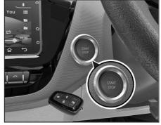
Start/Stop button is provided on the dashboard towards the left side of steering wheel.
