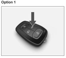
To release the tailgate, press the tail gate button on the remote.
