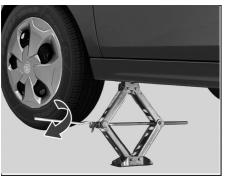
Lifting the rear wheel using jack
