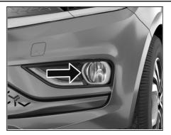
It turns 'ON' when the front fog lamp switch is pushed in with ignition 'ON' and position and parking / head lamp is 'ON'. An indicator on the switch will be illuminated when the front fog light is 'ON'.
