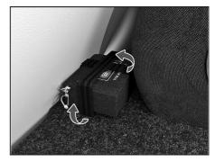
Remove the two Velcro as shown in figure and take out the puncture repair kit.
