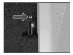
Pull the lever located at right side below near to driver seat to open the tailgate.
