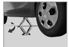
Lifting the front wheel using jack Remove wheel nuts with the help of wheel spanner and take out flat tyre.
