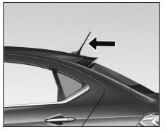
Antenna is located on the roof. Turn the antenna anticlockwise to remove it from the vehicle, if required.
