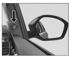
To fold / unfold the ORVMs, keep the Selector switch in center position (i.e. neither 'L' nor 'R, position) and then toggle down. This will operate when the ignition switch is in the "ACC" or "ON" position. Option 4: Rear View Mirror with Joystick Knob
