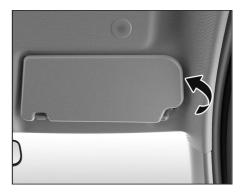
A pocket is provided on the back of the driver side sun visor to keep cards, papers, etc.
