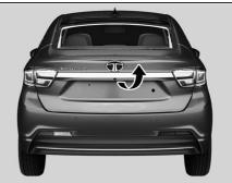
Press the tail gate opening button once (4) to unlock the tailgate with in authentication range (vehicle vicinity) of Smart key, then user has to press the tailgate switch within 30 sec.
